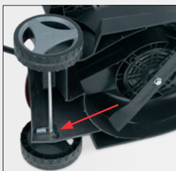
adjustable cutting height
